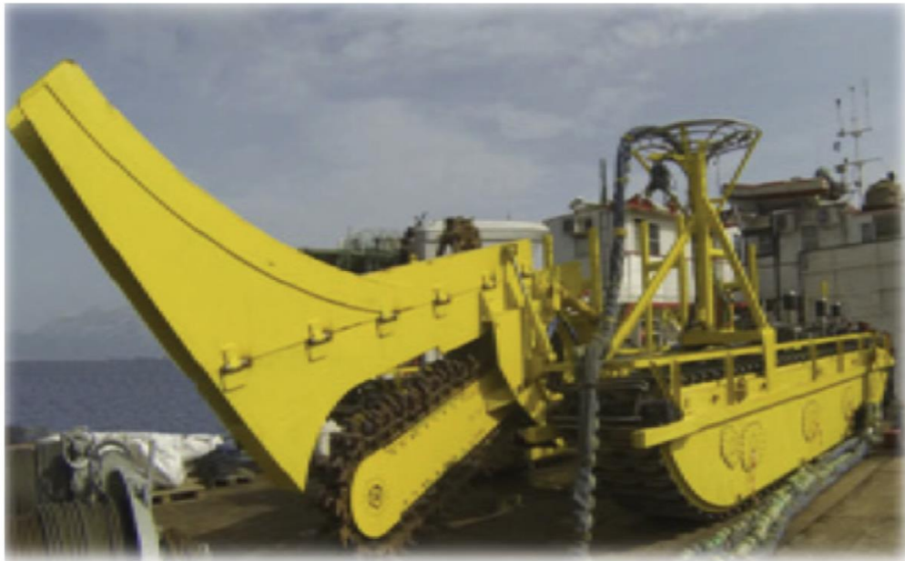
Fig. 13 Real chain cutter trenching machine owned by Assodivers
